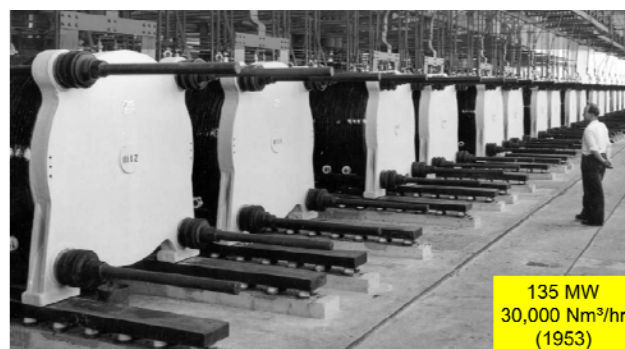
Figure 3. Electrolyser (multi-)stacking scale-up approach (top), with an historical example (bottom).
