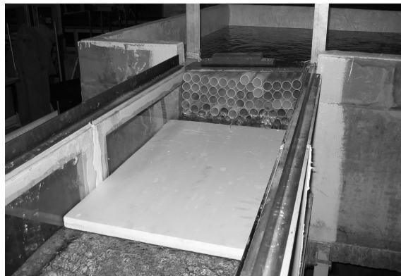
Figure 5.2. Floating panel at the upstream end of the flume
