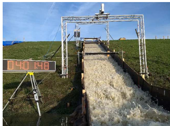
Figure 6. Left: side view of test location; right: test section during overflow test (source: Stephan Rikkert).
