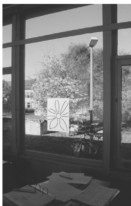
Figure 4: On site, full-scale test to define the adequate high of the horizontal stripe made of juxtaposed blue patterns.
