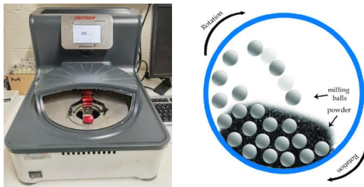
Figure 8. The ball milling machine used in the work of this thesis. Left: Fritsch Pulverisette P7, Right: schematic view of motion of the ball and powder mixture. 2
