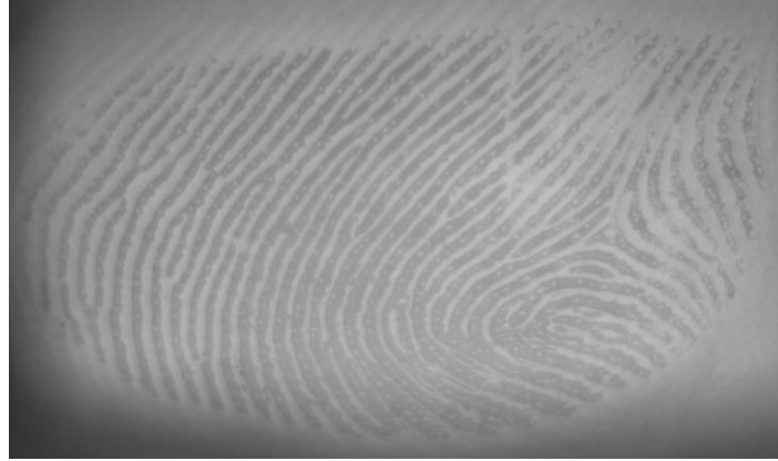
Fig. 1.11. Typical image of the fingerpad. Note that the ridges are black as they are in contact with the glass. The sweat pores are also visible (white points on the ridges).
