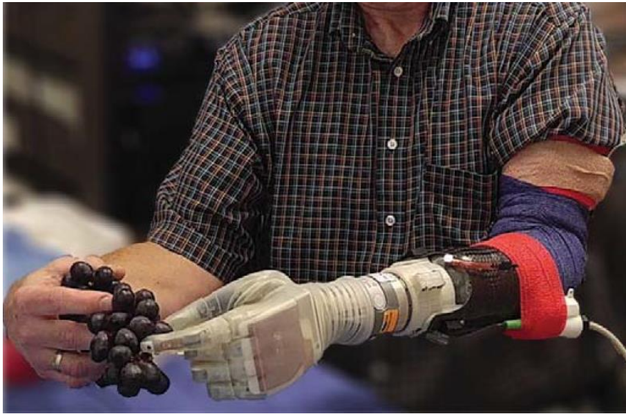
Fig. 5.2. A patient picking grapes with the DEKA LUKE arm. The DEKA Luke arm is a six-DOF bidirectional neuromyoelectric prosthetic hand and wrist that conveys biomimetic sensory feedback and is activated using electromyographic recordings from residual arm muscles. Adapted from (George et al., 2019).
