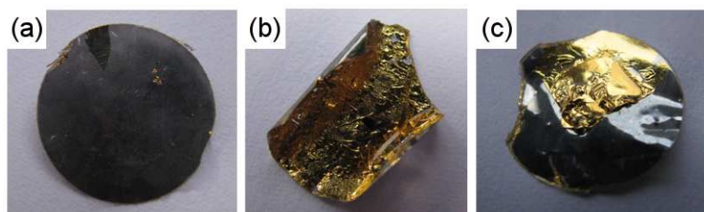
Figure A.4 Pictures of the evaporated gold layer after the process for different diameters: (a) 30 nm, (b) 70 nm, (c) 100 nm. For each of the three samples, the underwent treatment was as follows: soaking in methanol (10 min) and soaking in de-ionized water (10 min) (x3).
