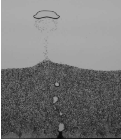
Fig. 9: Bubble carrying on grains in its wake for I = 6.5 mL/min and h_g = 4.5 cm at t = 19.5 s.
