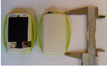
Fig. 3. Package containing a x-IMU MARG sensor and a battery. One side is equipped with Velcro for fixing.
