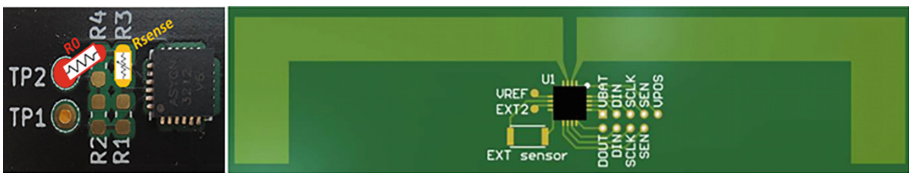
Fig. 3. On the left, half bridge employed to simulate the sensor behavior ( R_0 = 27 \text{ k}\Omega , R_{\text{sense}} = 22 \text{ k}\Omega , 33 \text{ k}\Omega ); on the right, the Asyn AS3212 RFID chip.
