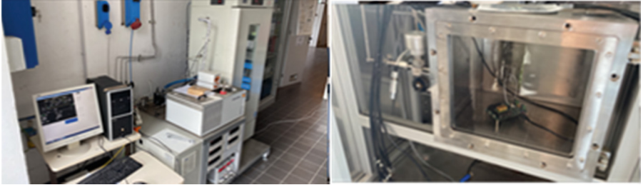
Fig. 1. Photos of the gas sensor characterization setup, including the 15 L large volume test chamber (LVTC) and associated equipment.
