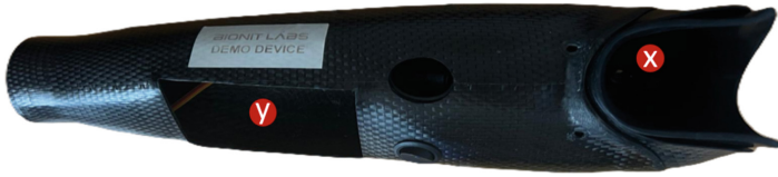
Fig. 4. Actuator placement on the prosthetic socket: Y indicates typical electrode locations; X denotes the area housing the residual limb.
