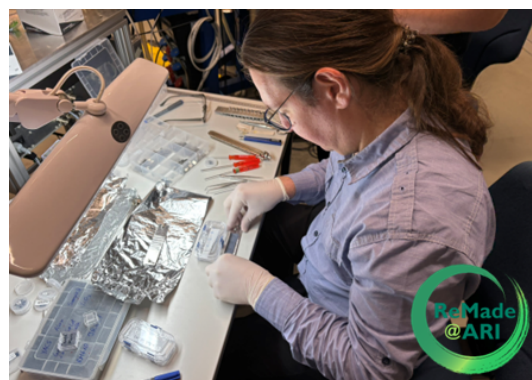
Fig. 3: Mounting of the Si stripes and masks.
