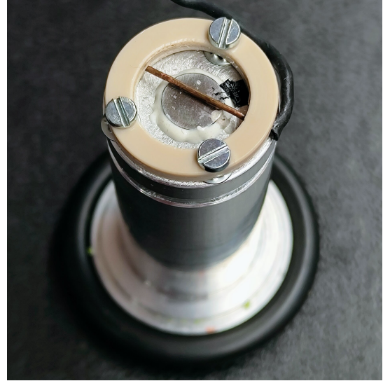
Fig. 2: A photo of the gas ionization counter showing the anode wire holder and the stainless-steel plate.
