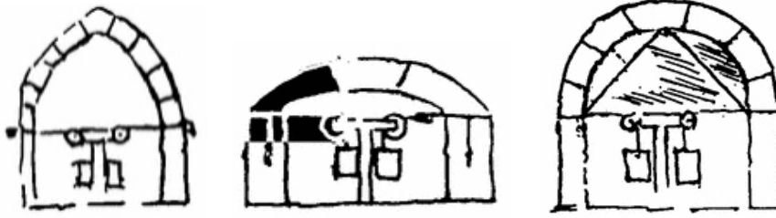
Figure 5.26 – da Vinci's intimations for an experimental estimate of the thrust on the abutment piers [BENVENUTO1991]
