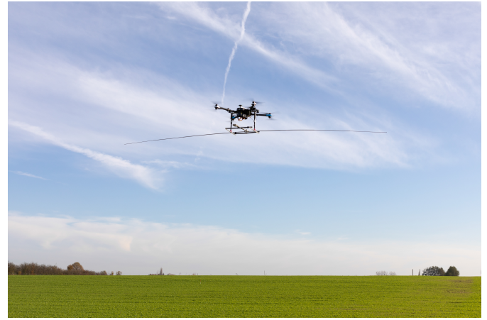
Fig. 8. Prototype of the drone-borne 15–45-MHz GPR for soil electrical conductivity mapping.
