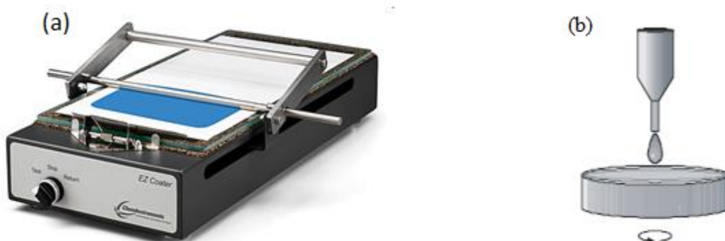
Figure 2: Illustration of (a) the bar coating and (b) the spin coating processes mainly used for deposition of our polysilazane sol-gel coatings.
