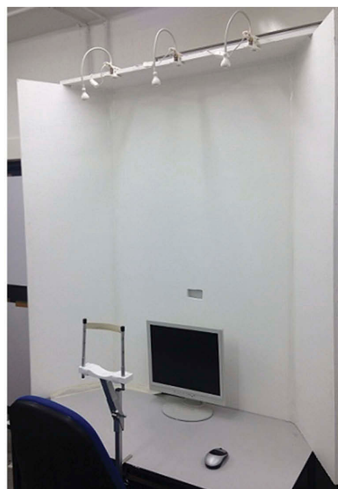
Fig. 1. Plan layout and photograph of the lighting chamber used in this study. Note that extraneous laboratory lighting (switched on for this photograph) was switched off during the tests, meaning that the room was dark other than the glare source, the VDU, and its surround.
