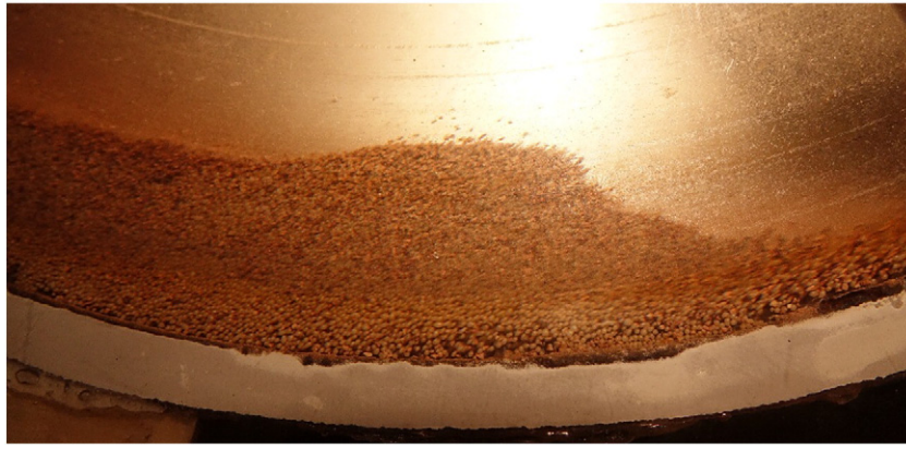
Fig. 9. “Snapshot” of a slug during low solids inventory. The solids are moving from right to left. A segregation of the cork (inner bed) and HDPE (outer bed) is observed.
