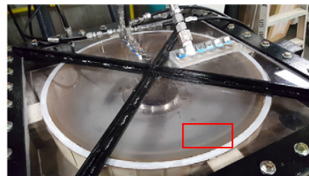
Fig. 6. Image of the slugging phenomenon. Slug at the front of the chamber (left), and slug at the back of the chamber (right). The red box on both images represents the Interrogation window used in the video analysis.
