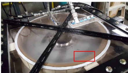
Fig. 6. Image of the slugging phenomenon. Slug at the front of the chamber (left), and slug at the back of the chamber (right). The red box on both images represents the Interrogation window used in the video analysis.
