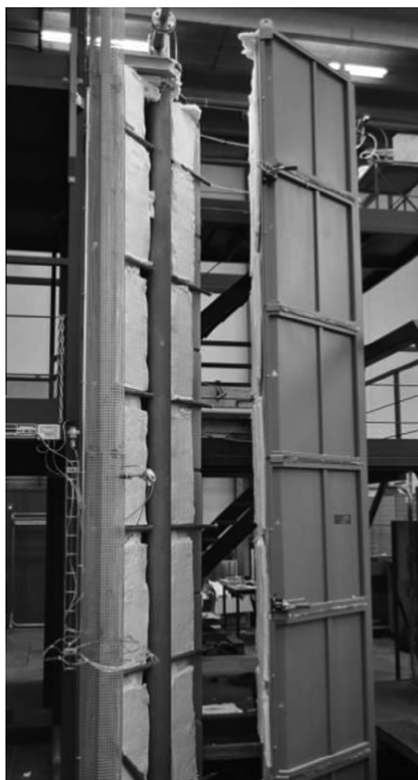
Fig. 3. LABORELEC–UCL drop tube furnace, with opened electrical modules, in order to access the vertical tube [5,12].
