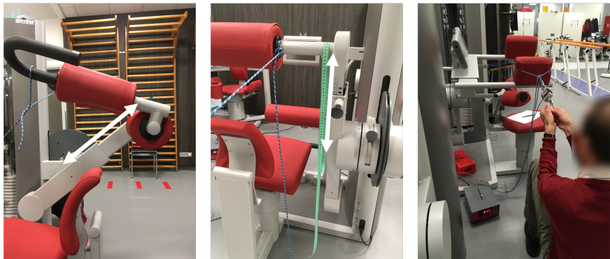
Fig. 6.2 Lever arms (white arrows) reported for the (Left) flexion and (Middle) extension devices. (Right) Calibration for the forces to apply in the model – example on the lateral bending device.
