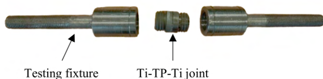
Figure A.4 Ti-TP-Ti weld and the fixtures in which they are mounted to perform the butt tensile tests.
