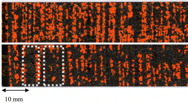
Figure 5.8 Optical micrograph of the fracture surface of a co-cured composite joint with 17.2 kg strong fishing lines spaced by 2 mm (orange strands). The grey regions correspond to zones with a limited number of fishing lines acting as bridging ligaments.
