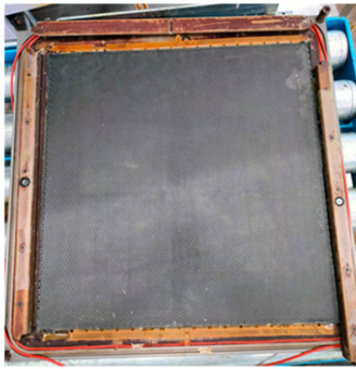
Figure 6B.4 Step 4 – Composite panel after opening the mould.
