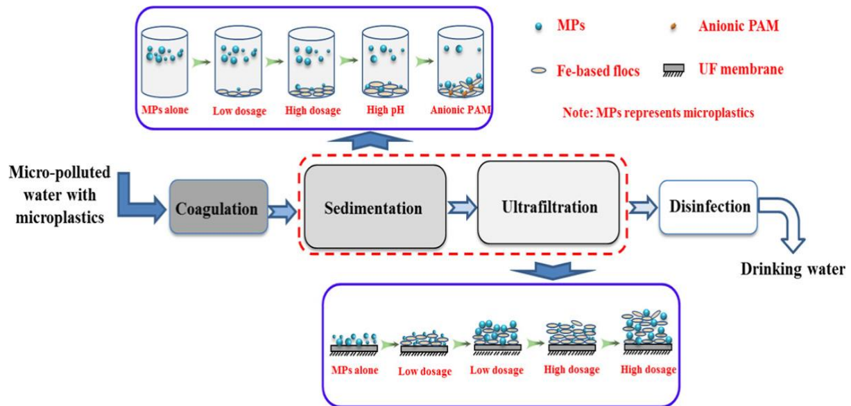
Fig. 6. Coagulation and ultrafiltration process for MPs removal. Reproduced from (Ma et al., 2019a) with permission from Elsevier.
