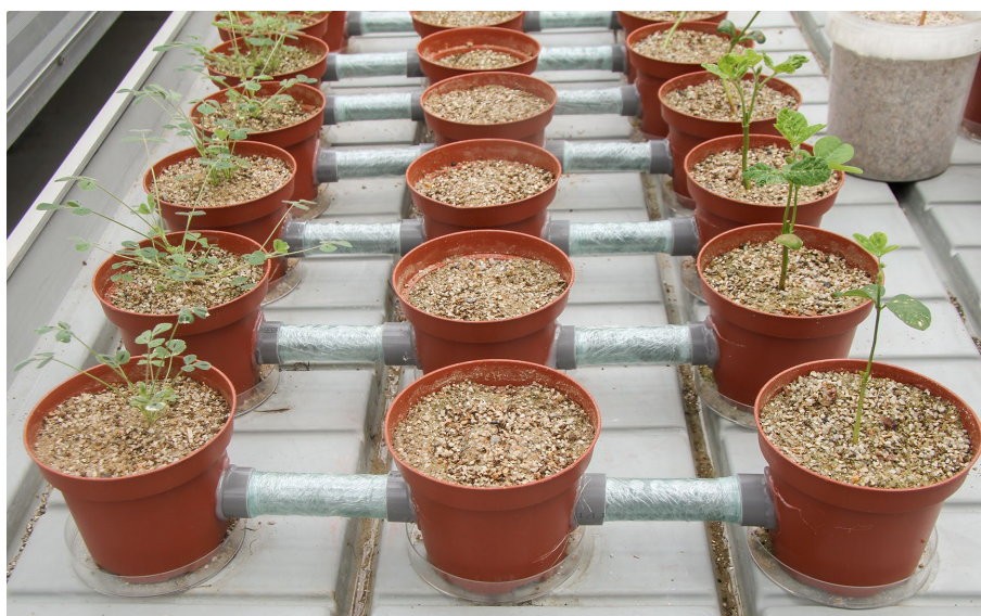
Figure S20. Picture of the three-compartment pot system.
