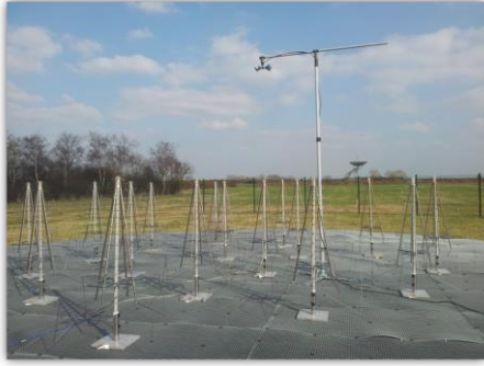
Figure 1: AAVS0 array at Lords Bridge Cambridge and telescopic mount holding the source antenna for the near field pattern test.
