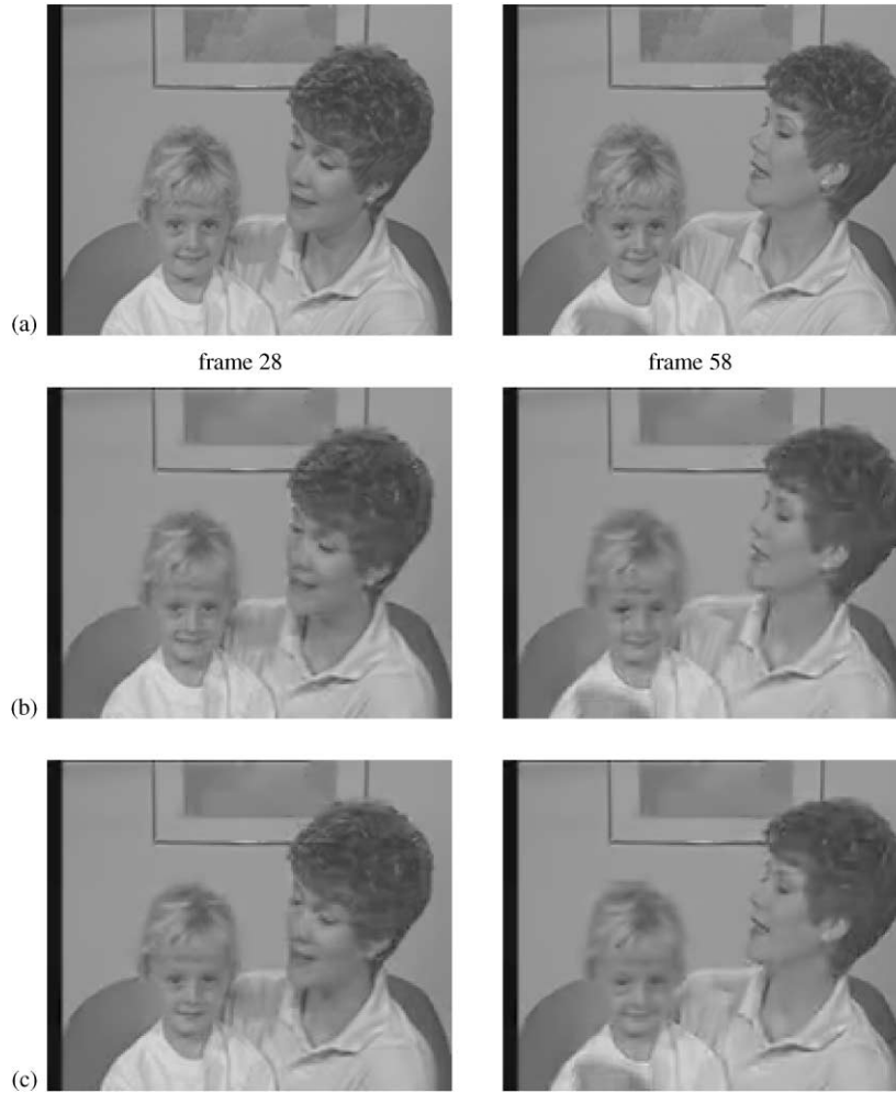
Fig. 9. “Mother-and-daughter” sequence (28 kbits/s, 10 frames/s): (a) original, (b) without perceptive considerations, (c) with block categorization according to masking capabilities during search window selection.
