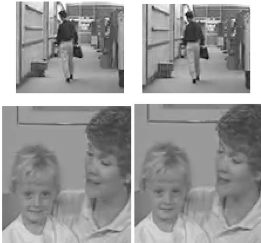
Fig. 10. Blow-ups of encoded frames. Left: encoded without perceptive consideration. Right: encoded with masking capabilities estimation. Top: “Hall-monitor”, frame 77. Bottom: “Mother-and-daughter”, frame 28.
