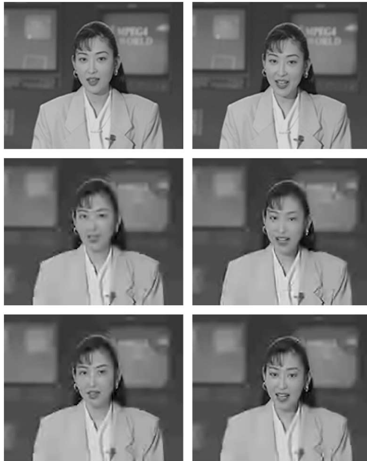
Fig. 2. Content-based bit-allocation for Akiyo video sequence. Frames 21 (left) and 77 (right): original (top), classic encoding (middle), subjective encoding (bottom).
