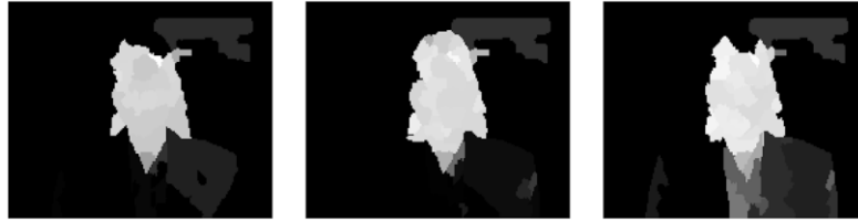
Fig. 1. Interest mask extracted for three successive coded frames of Akiyo (13, 17, 21). Lightning is proportional to the level of interest.
