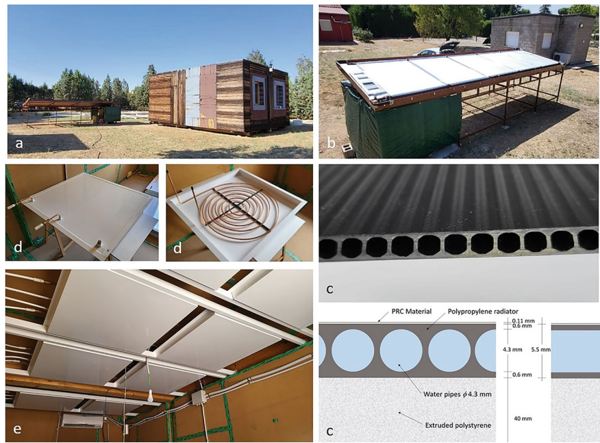
Fig. 2 a The full-scale experimental setup with two twin test cells, b sky radiators with PRC material, c cross and longitudinal sections of the sky radiator, d top view of an RCM with its connections to the heat exchanger, e array of RCMs as roof panels in the experimental cell
