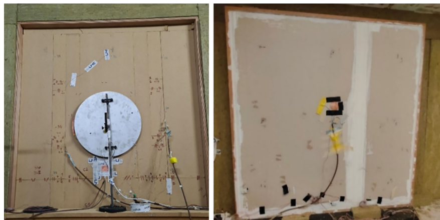
Fig. 3 Wall installed in the Rebecca climatic chamber (left cold side with the prototype, right hot side)
