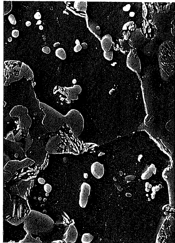
Figure 5.3: SEM micrographs of the typical microstructure of steel LSi after the 3 different heat-treatments; (a) specimen IV, (b) specimen V, and (c) specimen VI.
