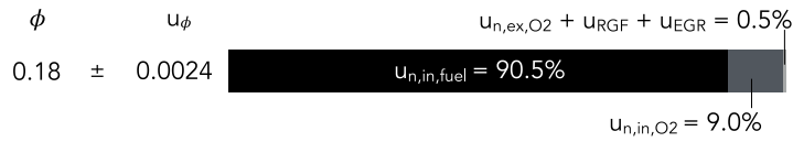
Figure A.30 – Equivalence ratio uncertainty breakdown for a low equivalence ratio run, without EGR, and with a combustion efficiency of 99.2%. The most impacting component is the fuel uncertainty itself, and the RGF is not impacting given that the unburned molecules are neglected for the computation of the equivalence ratio.
