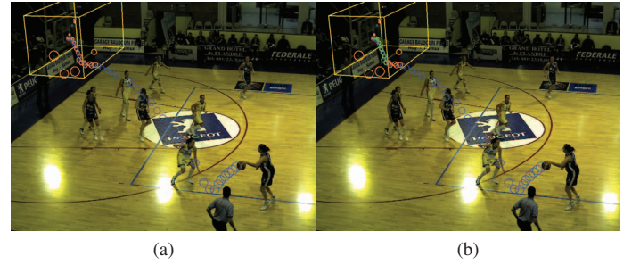
Fig. 2: (a) Ball candidates after spatial template matching (in orange) and ground truth (in blue), (b) Ball candidates classified as ballistic (in green) and non-ballistic (in orange) by temporal analysis.
