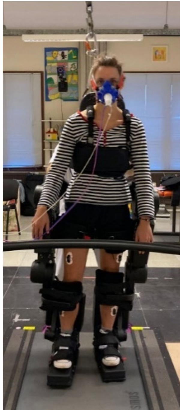
Figure 1. Illustration of a subject walking with the Atalante ® robot on the instrumented treadmill.
