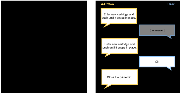
Figure 5: The application switches to a voice interface if the camera is covered. (Spoken texts were added to screenshot)
