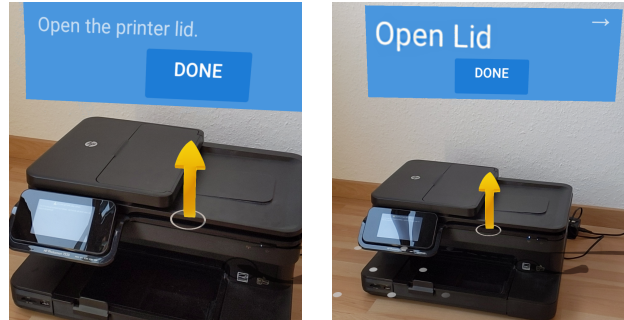
Figure 6: When the user moves away from the printer, the level of detail in the text on the window is decreased.
