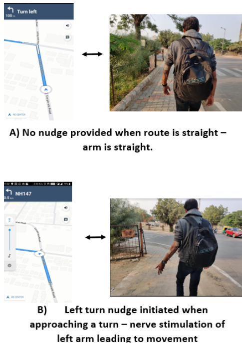
Figure 2: Navigation Nudges using our app and our hardware interface when user approaches a turn
