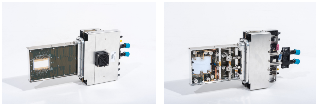
Figure 13. Picture of an assembled station looking at the sensor side (left) and at the cooling side (right).
