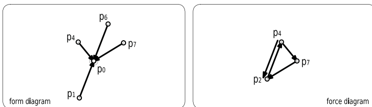
figure 95 a force network that is not in static equilib- rium.
