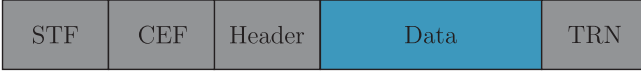
Fig. 1. 802.11 ad frame structure. TRN field is an optional overhead to enable beam-tracking.
