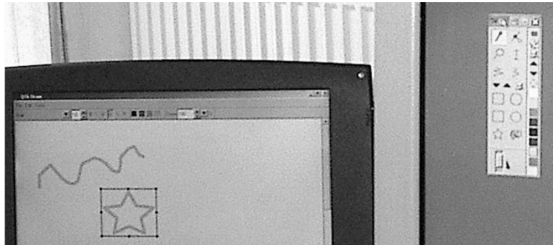
Fig. 9. Detaching the toolbar and the color palette from a TabletPC and attaching them together on a desktop (picture of situation in Fig. 8)
