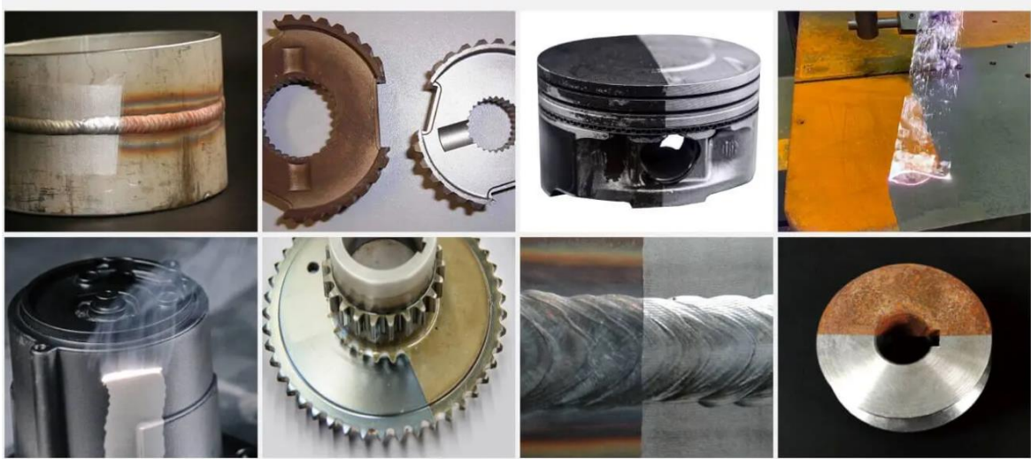
Examples of laser cleaning on metallic components ( www.hq-star.com )
