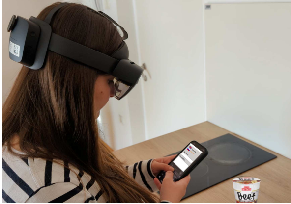
Fig. 3 A user wearing the HoloLens HMD with ARText prototype and holding the mobile device for text input.
