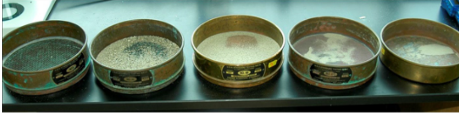
Figure 1.5: Separate sieves that have different sizes. They can be piled up in order to separate the sediments of different sizes. The sieve with the smaller mesh size, that contains the smaller sediments, is on the right of the picture. Courtesy of Joe Kistel from the "Think It Sink It Reef It" non-profit organization.
