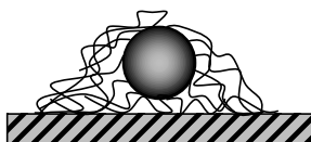
Figure 4.4: Schematic picture of the micellar structure for AFM characterization.
