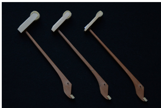
Figure 3.2: The three hammers (for bass, medium and treble notes) used in the experimental set-up.
