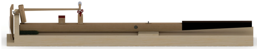
Fig. 1 The Viennese action of Johann Andreas Stein was used by Mozart and his contemporaries. A virtual 3D representation of the action is used to visualize the simulation results
