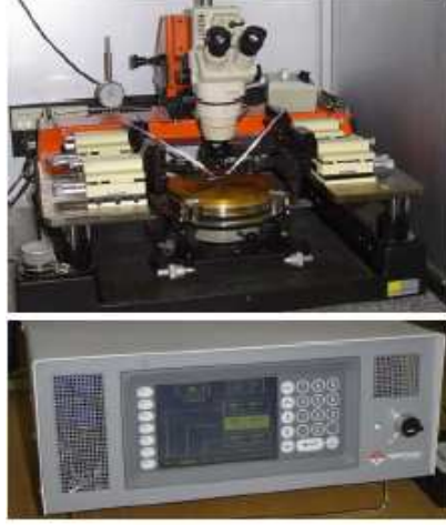
Figure 3.9: On-wafer probing station.
