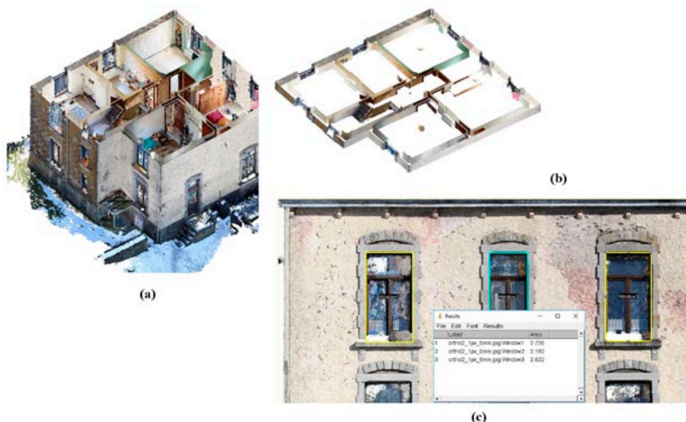
Figure 9. Building A surveyed with MVP: (a) model obtained by combining the interior and exterior reconstructions; (b) a cross-section through the whole-building 3D model; (c) drawings and measurements using an orthomosaic photo as support.
