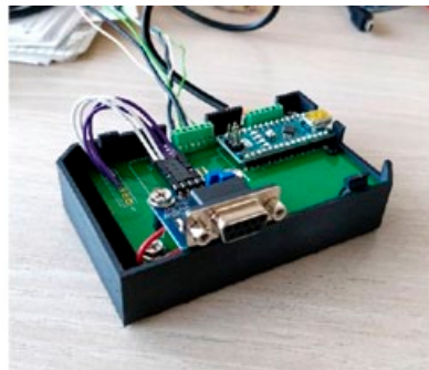
Figure 7. A tailored signal processing unit (open-source) to allow the measurement of heat flux.
