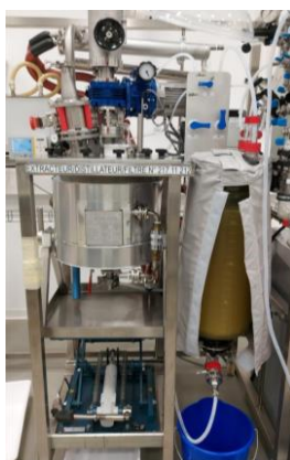
Figure 1.2-1 The 20 L Pignat pilot plant extractor used for the extraction of 850 g of untreated BSG
