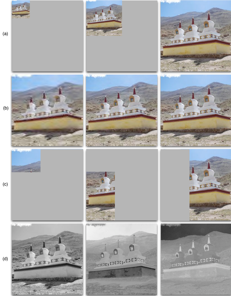
Figure 2.2: Scalability in JPEG 2000. Starting from a JPEG 2000 code-stream, image information can be extracted in several different ways: (a) by resolution, (b) by quality layer, (c) by spatial location, (d) by component (here: Y, Cb and Cr components, represented with a grayscale colormap).
