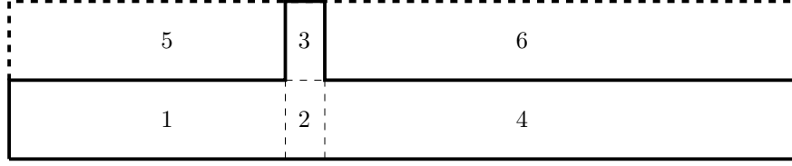
Figure 2.3: Illustration of the domain decomposition that is performed in our numerical simulations. The thick dashed lines show the original rectangular domain and the black solid lines show the resulting computational domain after the domain decomposition. The thin dashed lines show the interior boundaries between sub-domains.
