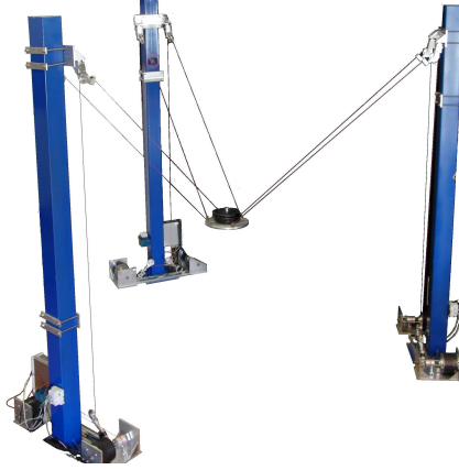
Figure 1: Fatronik/LIRMM prototype of a 3-meter-side 6-cable robot.
