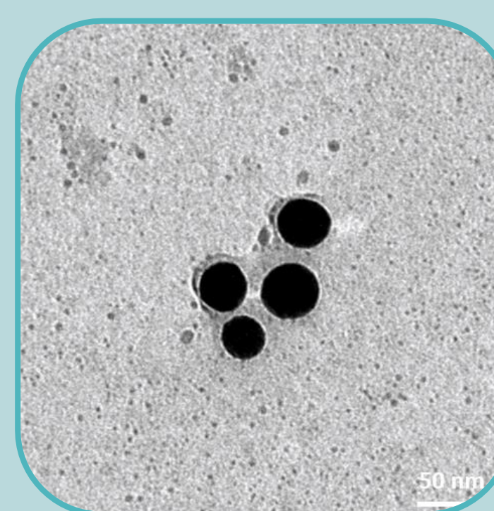
Good coating of gold nanoparticles with phage proteins
