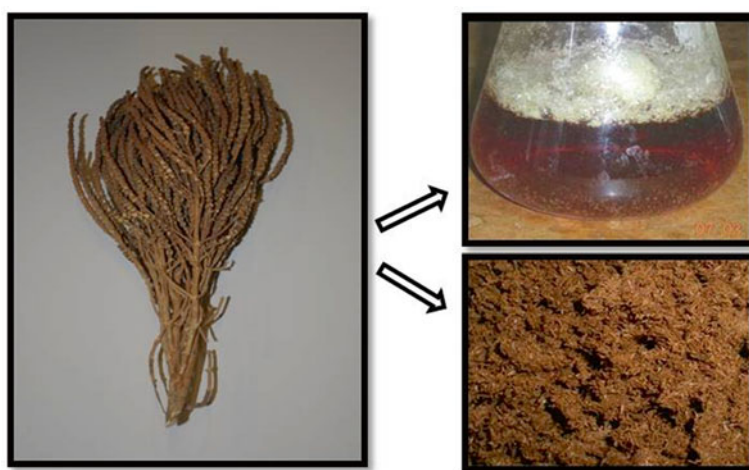
Fig. 2 Liquid fraction and digestible fiber fraction produced by pretreatment of S. bigelovii
