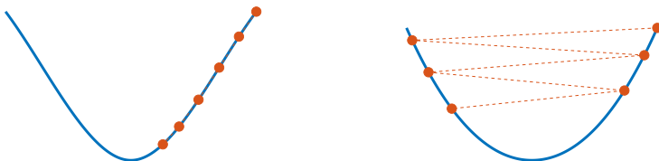
Fig. 10.6 N = 5 iterations of gradient method on f (left) and g (right) with step sizes h = \frac{2}{L+\mu} (left), defined in (10.80) and (10.81), and h = \frac{2.1}{L+\mu} (right) and |x_0 - x_*| = 0.42 , M = L = 1 , \mu = 0.3 .
