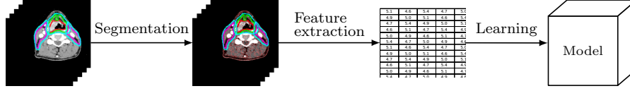
Figure 3.2 – The learning. The model is learnt from images with delineated objects. Homogeneous areas of the image are identified by the watershed algorithm (i.e. during the segmentation step). Features are extracted for each superpixel. The model, which is formed of the sequence and submodels, is learnt from the features.
