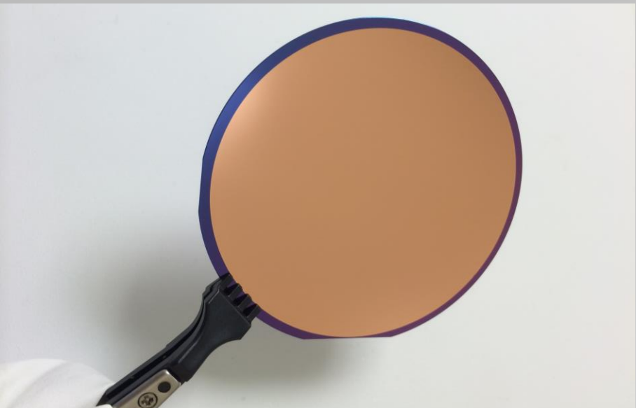
3 inch-Si wafer thermally oxidized and coated with a thin Cu film.
