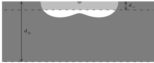
Figure 5.2: Layer of influence for the double-D head and for a response ratio \alpha = 0.95 . Vertical cut through the center of the head is illustrated and shows the projection of TX (—) and RX (---) coils, the border of generating volume (- · -), the positive (dark gray) and negative (light gray) layer of influence with corresponding positive and negative depths of influence d_+ and d_- . The holes in the layer of influence appear in white.
