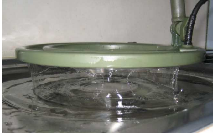
Figure 6.9: Typical water film appearing when lifting the head out of the water.
